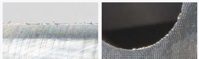
Before processing - Distinct burrs on the edge. Milling grooves on the surface.
