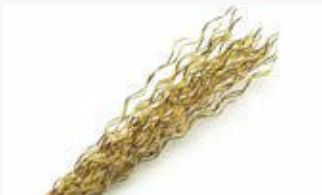
Brass-coated steel wire
